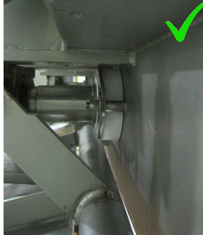
The drive motor is separated from the blender wall to prevent oil or grease from entering the blender.
